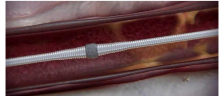
Diamond coated crown orbits in an elliptical path
